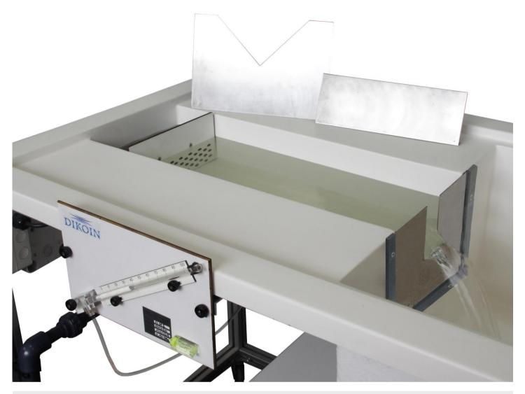
This is a set of 4 overflow weir plates with different shapes and functions. Plus an inclined tube manometer connected to the bottom of the channel to measure the water-flow height.
